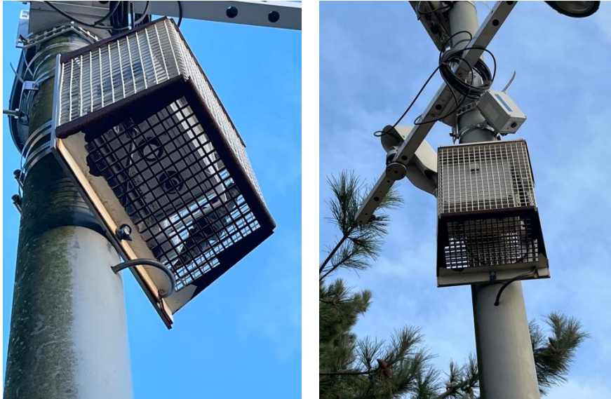
Figure 10: Aeroqual AQY1 supplied by Telensa, after 23 months of operation (photos: H Steventon)
