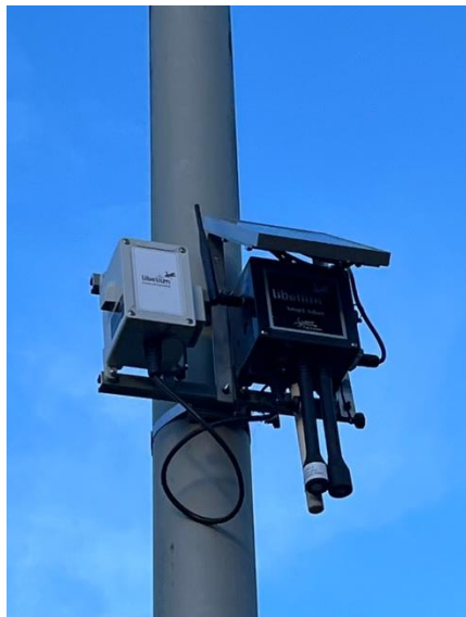
Figure 9: Libelium Air Quality Sensor supplied by SSE, after seven months of operation (photo: H Steventon)
