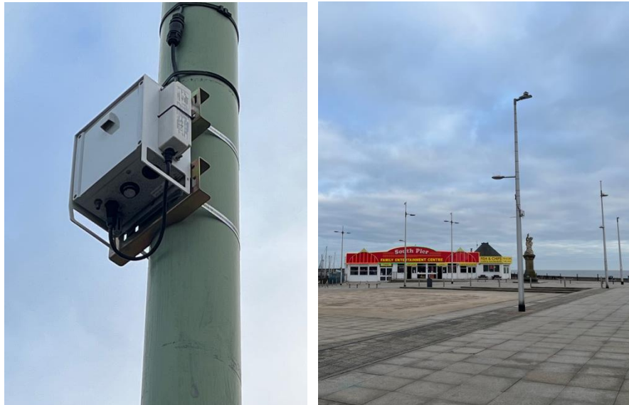
Figure 8: Aeroqual Air Quality Sensors supplied by CIMCON, after eleven months of operation (photo: H Steventon)
