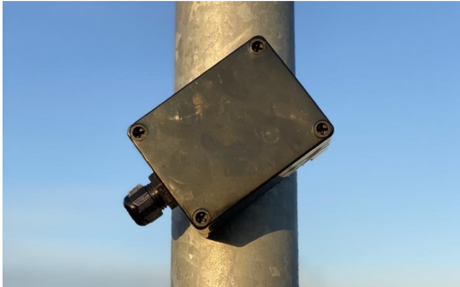
Figure 1: Uniotech on-column road surface temperature sensor, image from Michael Price, Uniotech, 16/12/2019
