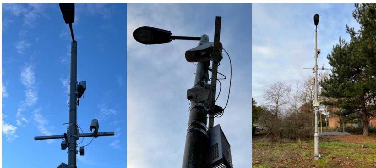
Figure 47: Vaisala RST sensor supplied by Telensa, campus location (photos: H Steventon)
