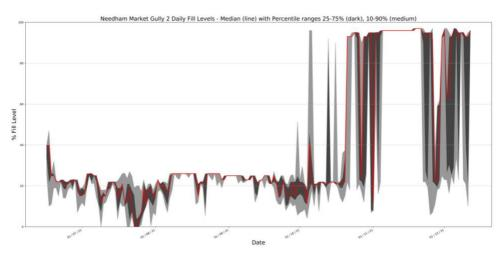
*Figure 12: Needham Market Gully 2 Daily Fill Levels - Median (line) with Percentile ranges 25-75% (dark), 10-90% (medium)*
