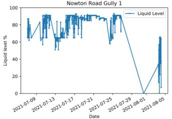
Figure 29: Reported liquid levels from sensor in Nowton Road Gully 1
