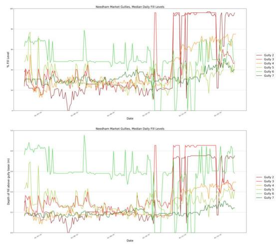
Figure 18: Median fill levels from north-west gullies, as percentage fill and depth of fill
