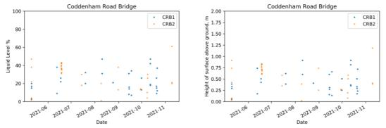
Figure 25: Apparent fill level as given (% liquid level) and converted to height of surface above ground level (m) for consecutive non-zero values only
