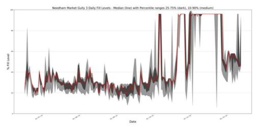
*Figure 13: Needham Market Gully 3 Daily Fill Levels - Median (line) with Percentile ranges 25-75% (dark), 10-90% (medium)*
