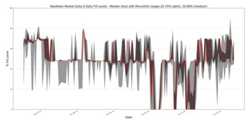
*Figure 16: Needham Market Gully 6 Daily Fill Levels - Median (line) with Percentile ranges 25-75% (dark), 10-90% (medium)*
