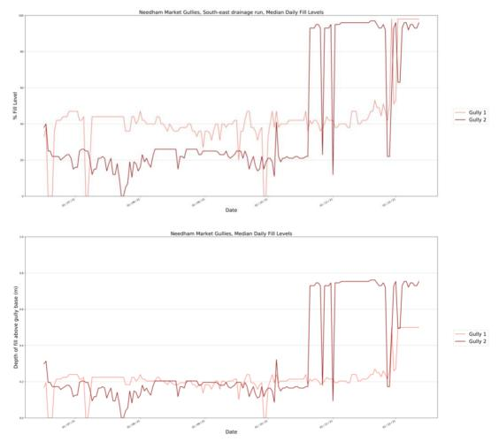
Figure 19: Median fill levels from south-east gullies, as percentage fill and depth of fill
