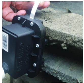
Figure 2: Danalto Gully Spy fitted to a gully at Adastral Park. Photo H Steventon
