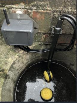
Figure 4: Map16 gully sensor, image from data sheet
