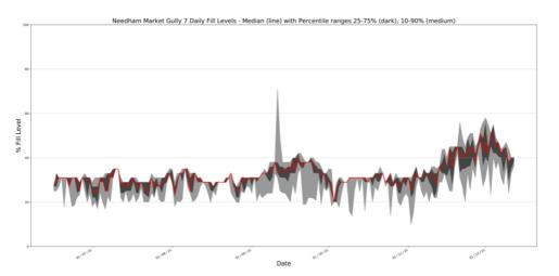
*Figure 17: Needham Market Gully 7 Daily Fill Levels - Median (line) with Percentile ranges 25-75% (dark), 10-90% (medium)*
