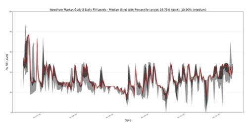
*Figure 15: Needham Market Gully 5 Daily Fill Levels - Median (line) with Percentile ranges 25-75% (dark), 10-90% (medium)*
