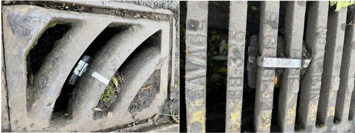
Figure 48: Photos of KaarbonTech sensors showing physical appearance after 6 months installation (photos: H Steventon)
