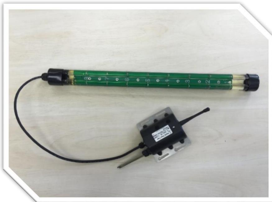
Figure 3: InTouch SmartWater Gully Smart sensor
