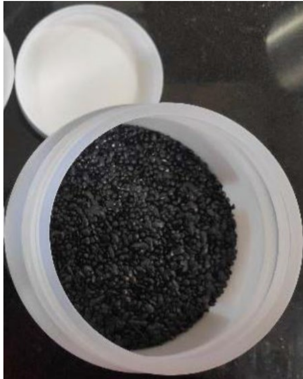
Figure 1-2 - Additive 4 sample before blending with bitumen using the wet process
