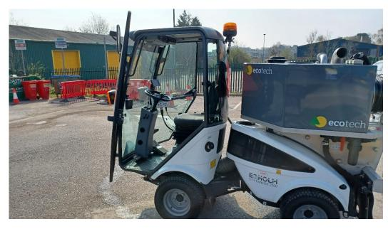
Ehgolm City Ranger 2260 used for trial. Illustrates size and compactness of the vehicle, including cabin, and also articulated steering arrangement.
