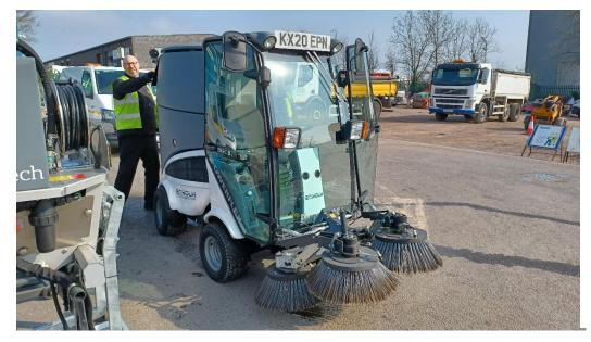
Front of vehicle with view of cabin housing, offering good panoramic visibility and also sweeper attachment.
