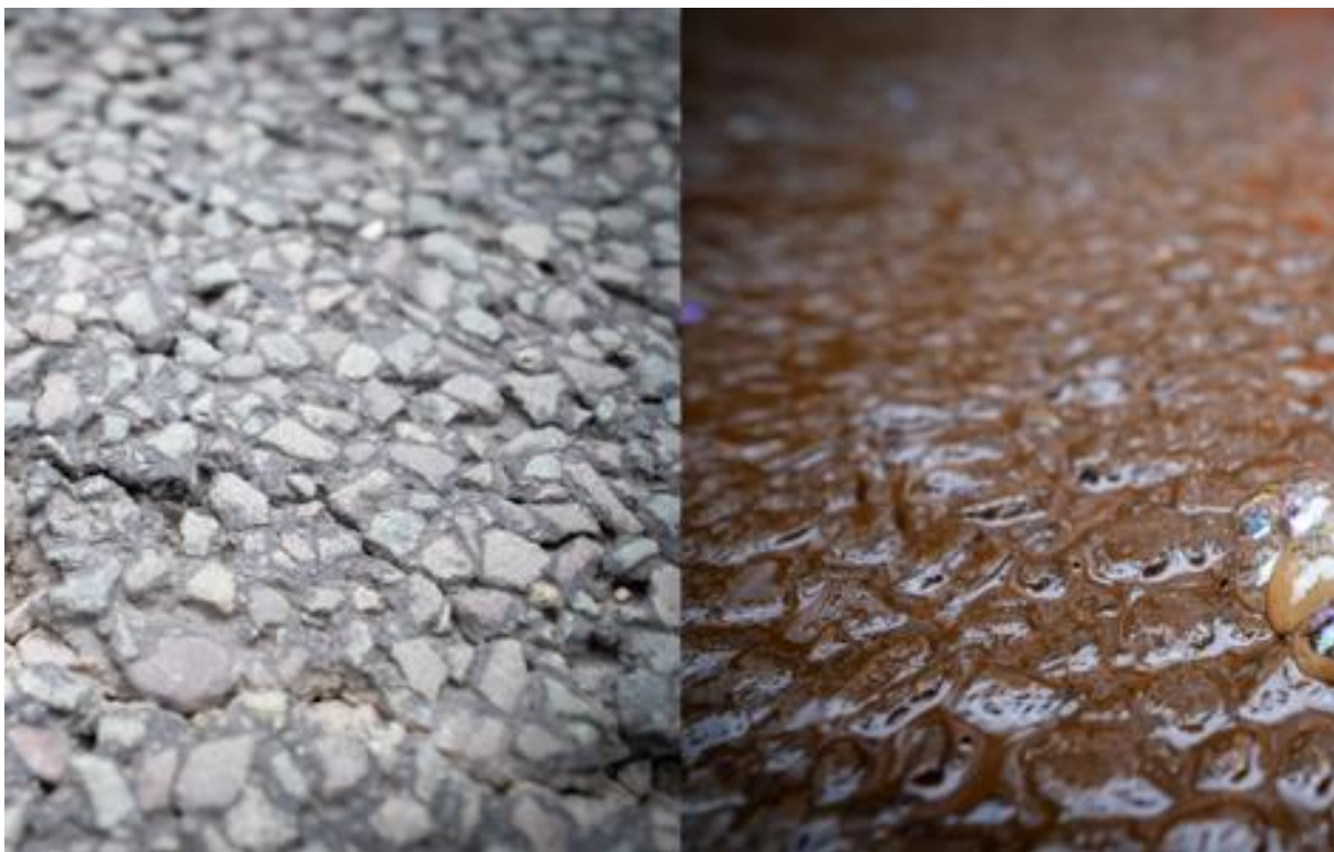
Figure 10 – comparison between untreated section (left) and section sprayed with asphalt rejuvenator during curing period (right).
