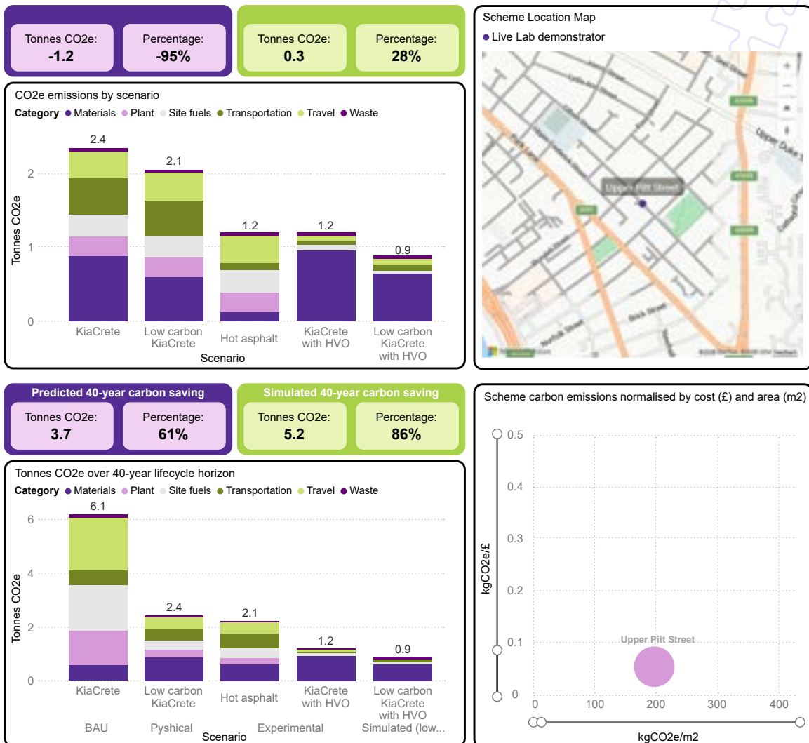
Figure 8: Carbon profiles (top) and 40-year carbon profiles (bottom) for KiaCrete scheme on Upper Pitt Street
