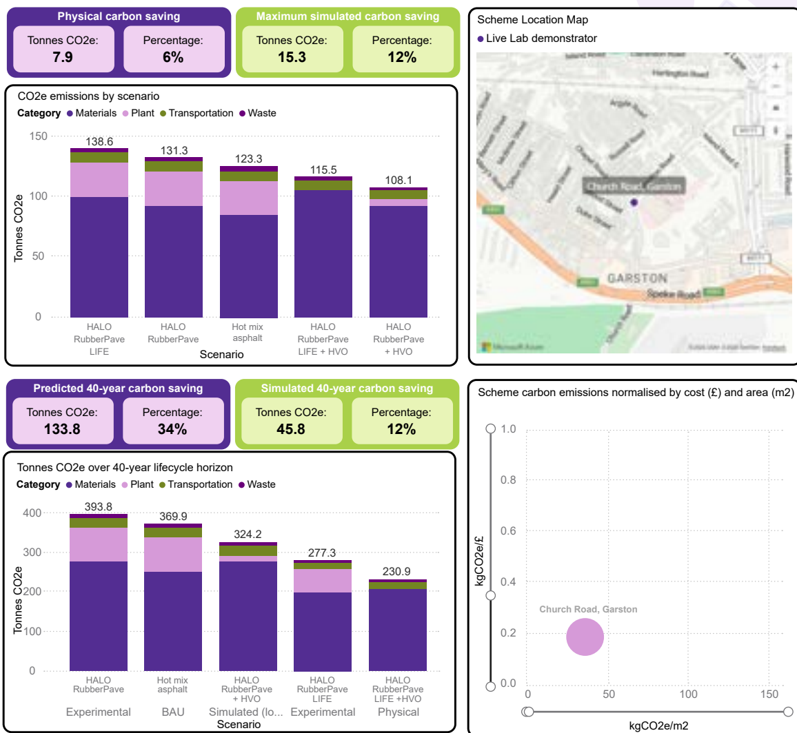
Figure 10: Carbon profiles (top) and 40-year carbon profiles (bottom) for RubberPave LIFE scheme on Church Road, Garston
