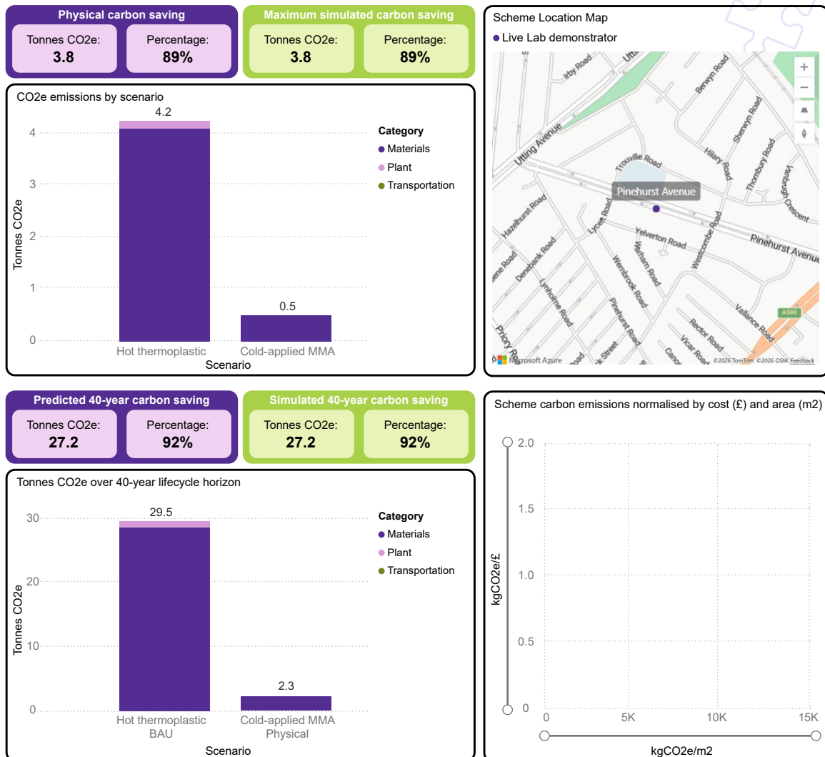
Figure 15: Carbon profiles for cold-applied MMA scheme on Pinehurst Avenue, including upfront emissions (top) and long-term emissions over 40 years (bottom).
