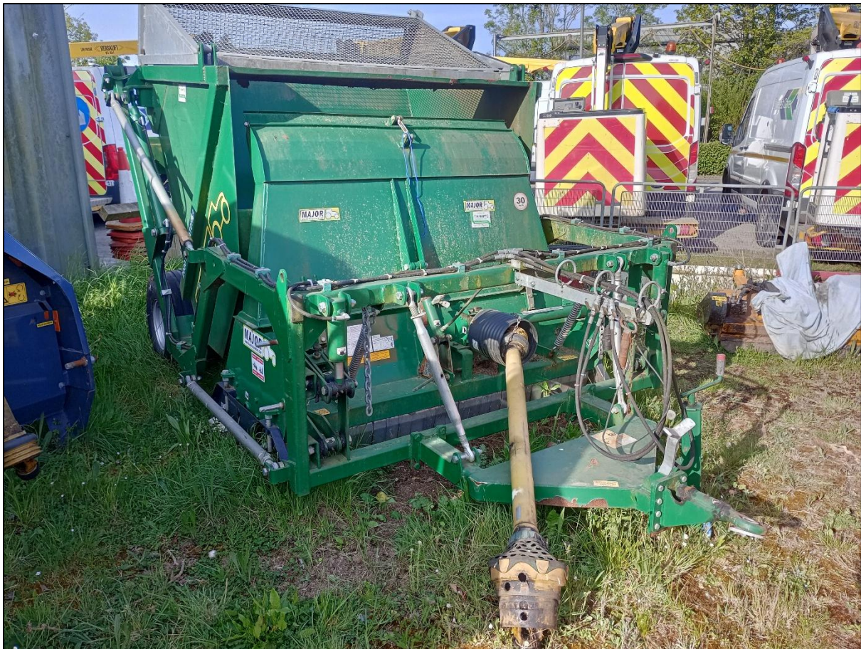
Major MJ2000 flail collector – used by SGC on the dual carriageway / B-road cut-and-collect trial
