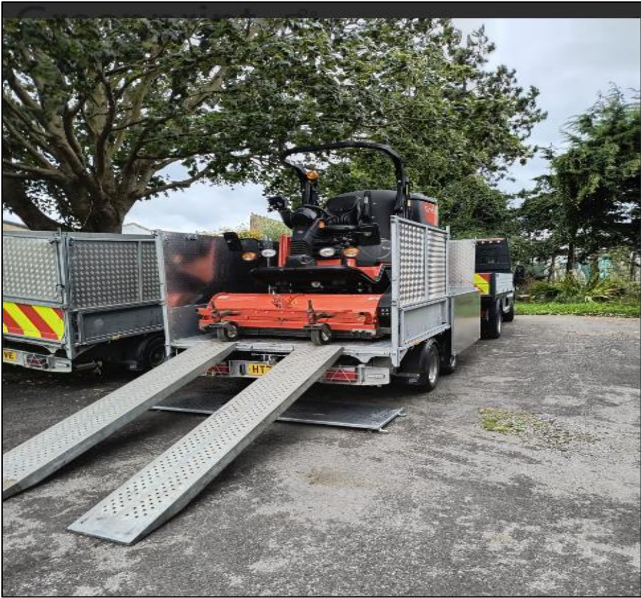
Tipping trailer – used to transport mower to site and transport cuttings back to depot
