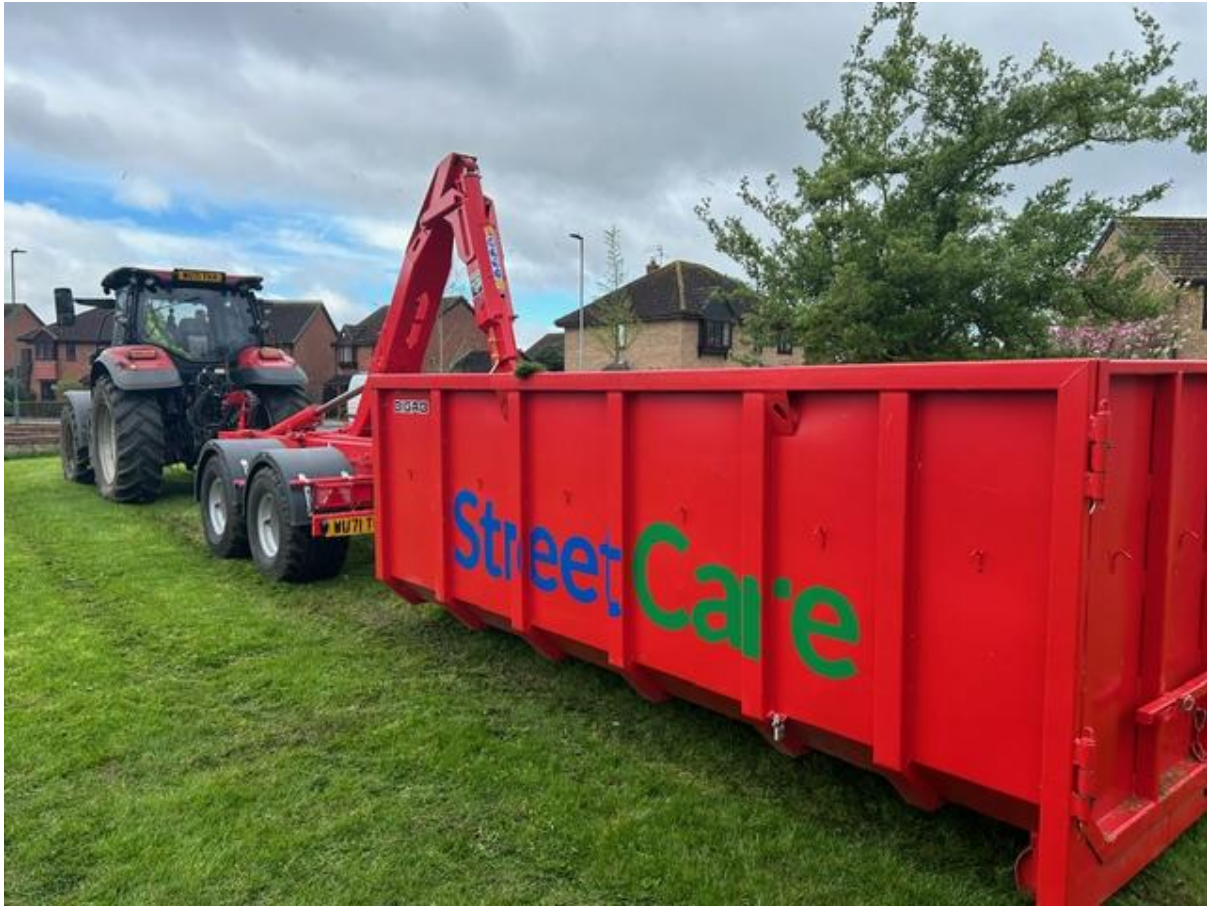
BigAb B12 hook-lift trailer & container
